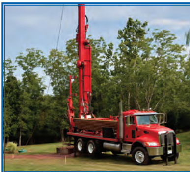
Rotary drill rig.
