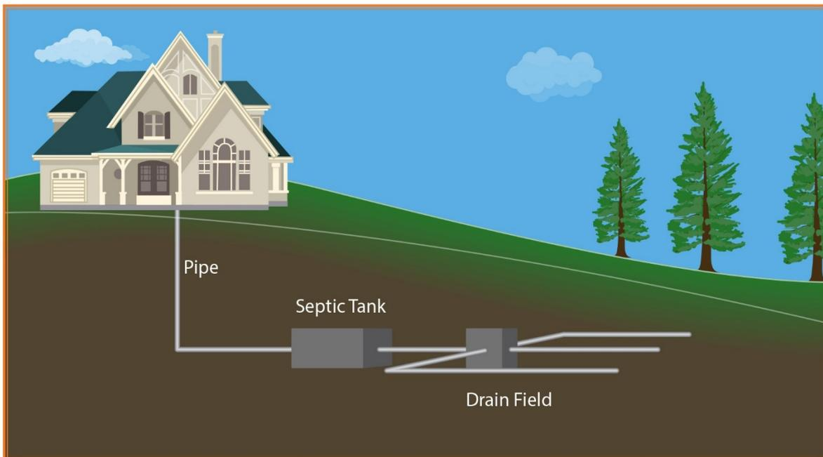
*This image is intended to represent some of the components that can be included in a septic system and is not intended as an installation guide. Check local codes for actual requirements and restrictions.*
